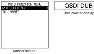
4 Press the ⇒ button to display the menu level 2 for the item "QSDI DUBBING", and select the dubbing data with the ↓ button.
